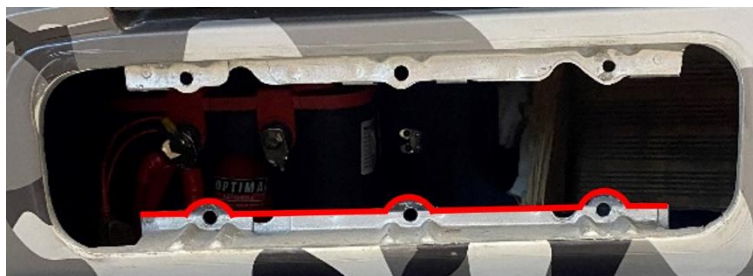
Figure 2: Cutting the valence so that the new lights can be installed. Red curve shows metal along the bottom that also needs to be trimmed.
